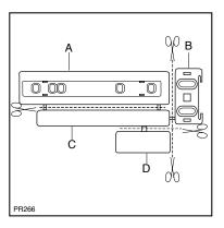
Place guide (A) on the inside part of the furniture door, upper and lower position as shown in the figure and mark the position of external holes. Having drilled the holes, fix the guide with the screws supplied.
